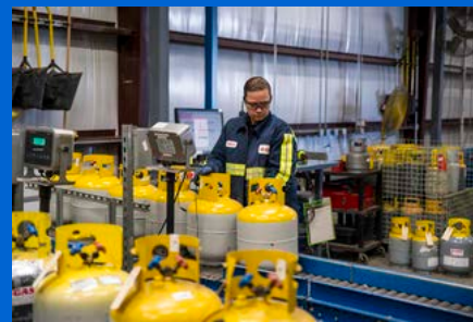
An A-Gas employee collects recovered refrigerant at A-Gas’ Rhome, Texas, plant. This is the first step in the reclamation process once the refrigerant cylinders arrive at the A-Gas plant. Photo credit: A-Gas.
